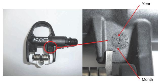
The date code on HM pedals consists of a letter (A through L) on one side on the bottom of the pedal body that represents the month, and a single number on the other side that represents the year, so that "L" and "5" on the pedal means it was produced in December 2005.
