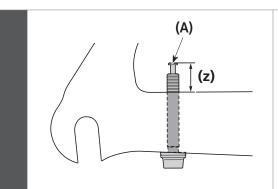
Insert the brake caliper mounting bolts C into the frame mount area, and make sure that the lengths of the protruding sections of the bolts are 13 mm.
