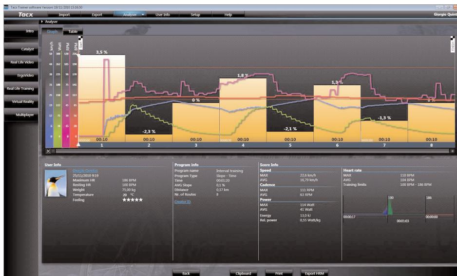
The horizontal axis shows distance or time. You can determine which data you want to see in the graph by ticking the axes speed, output, cadence and heart rate. The upper and lower limits of heart rate are shown as an interrupted horizontal line. The coloured field represents the course. Underneath the graph you will find data regarding the user and additional information.
